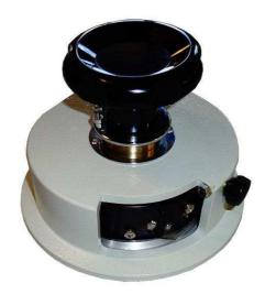
The BRANCA Circular Sample Cutter prepares circular samples of fabric, paper, plastic with 100 cm<sup>2</sup> of exact area. Together with an electronic scale the sample cutter is suitable to determine the mass per unit areas (m<sup>2</sup> or yd<sup>2</sup>).
